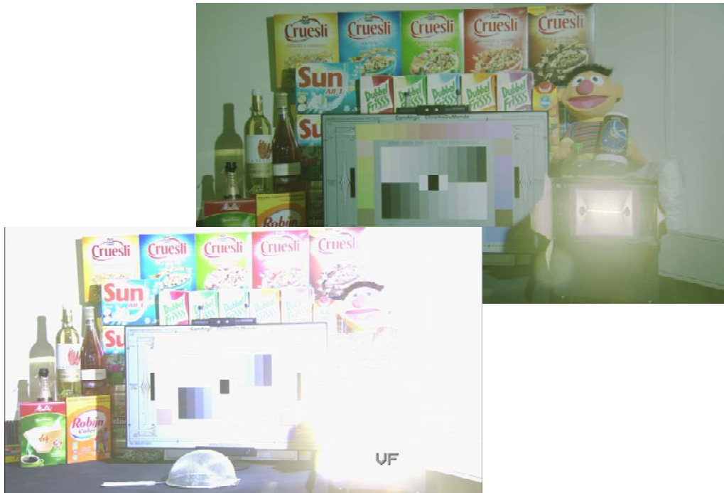
Figure 5 – Image down-left: normal operation, Image upper-right HDR image.
