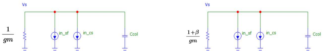
Figure 4: Noise small signal diagram. Left: reset-on, Right: reset-off
